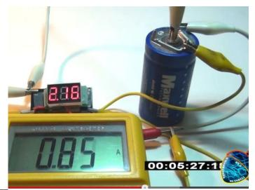
Above is supercap charging polarity. Charging wires are the two white wires. The bottom darker wire below is not a charging wire
