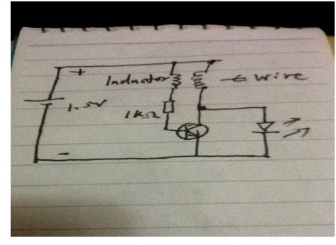
Instead of using a toroid,I wrap the copper wire 8 to 10 turns on the inductor as captured.
