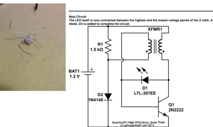
The addition of D2 represents an added drain of about 0.7mA, but aside from providing a return path to the LED, it also functions as a rudimentary power regulator by maintaining the voltage to the transistor's base just at its conducting point, regardless of input voltage. This allows the circuit to operate over a much wider voltage range, from 2-volts to around 0.9-volt with much better current (and brightness) regulation. As built, this circuit will operate down to just below 0.6v.
